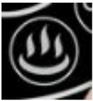
**The Heat button** is probably the most important button that is on the control panel. **YOU MUST** ensure that this is illuminated at all times. When the hot tub is heating it will glow red and when it is at the temperature you have selected it will glow green. If this is not illuminated the hot tub will lose temperature.
