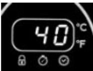
**Temperature Guide / lock notification** This panel shows the approx temperature of the water in the hot tub please note this is a guide only. The lock symbol will be illuminated when the control panel is locked.
