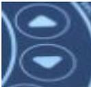
**The Temp Control Buttons** operates the temperature control adjust the temperature selection up and down the temperature will flash in the temperature guide window whilst you make your selection Please bear in mind if you increase the temperature the hot tub will increase by approx 2 c and hour depending on conditions.
