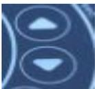
**The Temperature Control Buttons** operates the temperature control adjust the temperature selection up and down the temperature will flash in the temperature guide window whilst you make your selection Please bear in mind if you increase the temperature the hot tub will increase by approx 2 c and hour depending on conditions.
