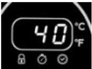
**Temperature Guide / lock notification** This panel shows the approx temperature of the water in the hot tub please note this is a guide only. The lock symbol will be illuminated when the control panel is locked.
